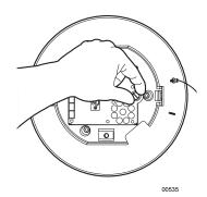
b. Turn the thumbscrew and open the hinged door to the back box. Pull wiring into the back box through the conduit fitting. Refer to Tables A and B in the Appendix for wiring distances.
